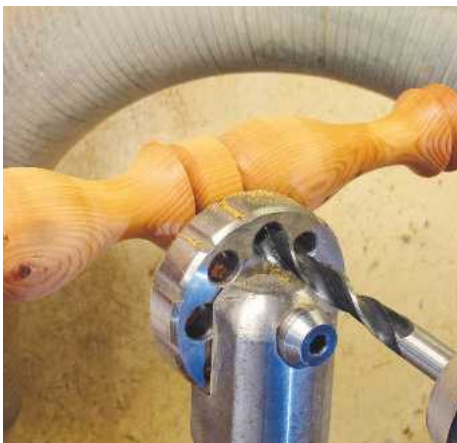
▲ Pic.25 Les is using the indexing on his lathe as well as a purpose-made drilling jig. He could have done it carefully freehand or using the banjo instead of the toolrest
